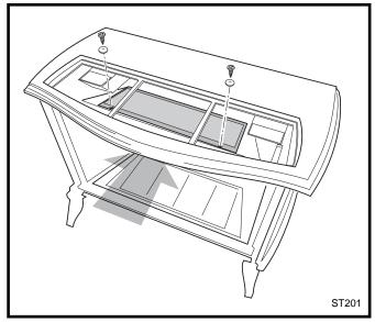
Fig. 37 Remove the catalytic combustor module.
